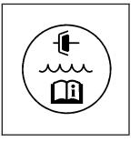
The hydraulic clutch fluid reservoir cap has this symbol on it. See *Engine Compartment Overview on page 5-14* for reservoir location.
